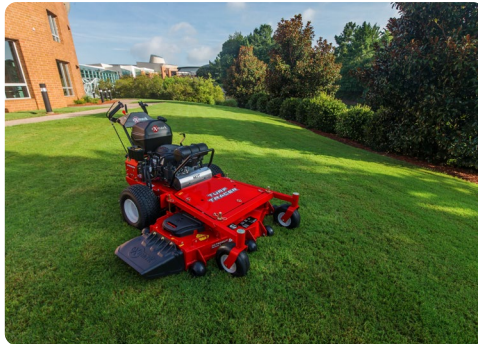
Exmark® Turf Tracer® with XiQ Technology, capable of mowing in manual or autonomous modes
