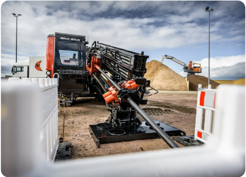
Ditch Witch AT120, world's largest all-terrain horizontal directional drill
