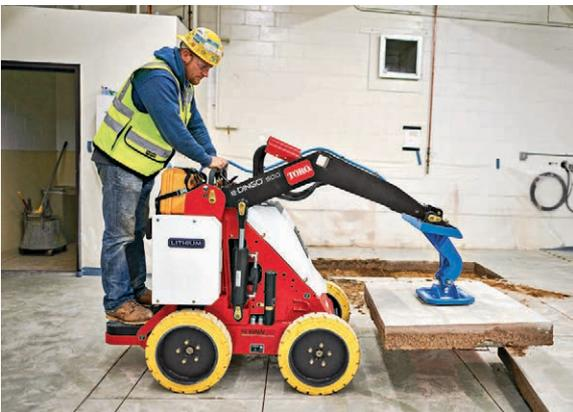
A major step for the electric-powered equipment market, Toro's **e-Dingo**® compact utility loader allows contractors and construction professionals to realize all the benefits and power of a standard compact utility loader with zero exhaust emissions. Ideal for indoor construction and demolition jobs, the lithium-ion battery powered e-Dingo has the ability to use common attachments that work with Dingo models, allowing operators to handle a wide variety of tasks with greater efficiency. ◀
