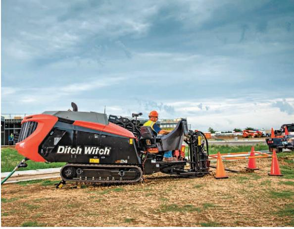
The Ditch Witch® **JT24** has defined the evolution of the mid-size horizontal directional drill market. Packing the power, durability and best-in-class stability, the JT24 is designed for fiber, gas and other utility installations in residential and urban areas. Operators can confidently traverse city curbs and uneven terrain, while still maintaining a small footprint and optimum power. ◀
